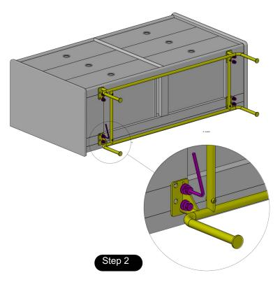
Install the metal feet and fix them with M8\*20 flat head screws. After the metal feet are installed, stand up the cabinet.
