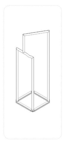
Secure the third-tier rack, base, and wooden foot pads, then tighten the joint between the second-tier and third-tier racks.
