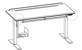
Connect the data cables and power cables of the lifts on both sides to the handles, turn on the power, and test whether the lifting function is normal.
