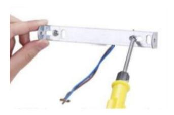
Drill holes according to the mounting base hole-spacing (8-12cm)
